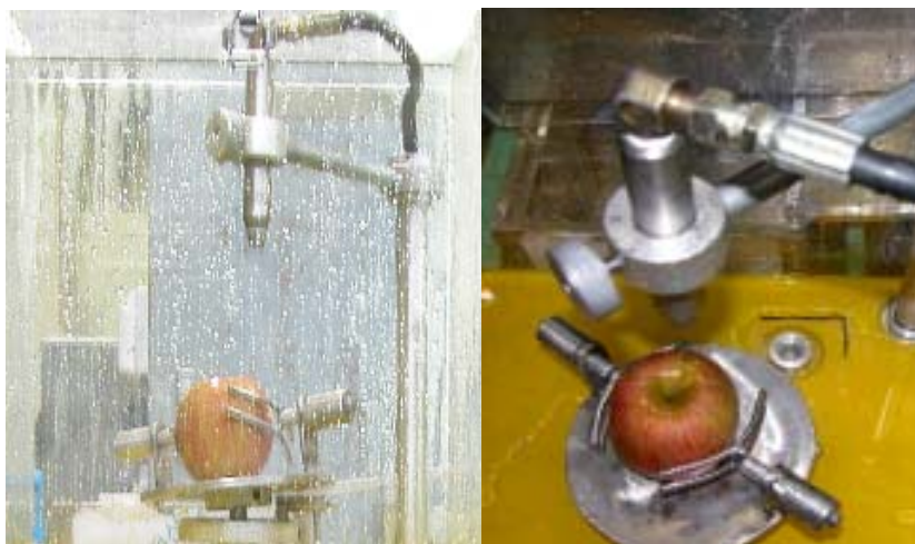
Fig. 3-7-4. Experimental apparatus of pressured mild hot water treatment system for apple
